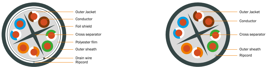
Cable view in a cross section
