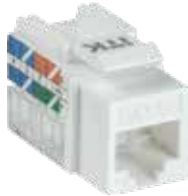
ITK Module Keystone Jack category 6A UTP 110 IDC 90 degrees CS1-1C6AU-11
